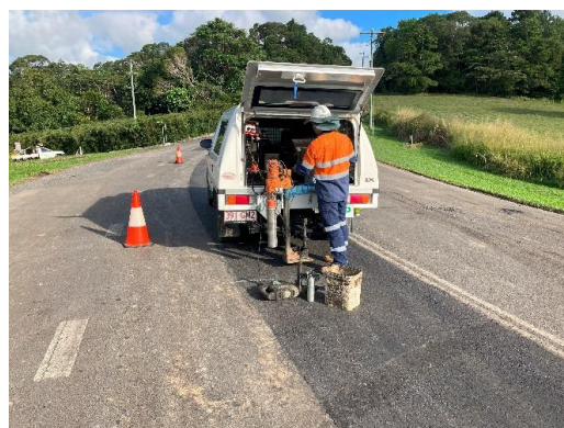
Asphalt density testing
