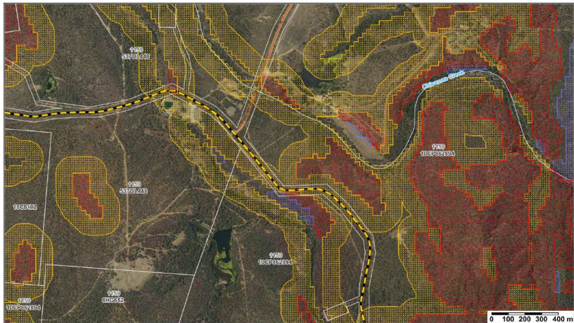
Figure 4-2: Bushfire Hazard Overlay Map showing Mullock heap 1 in the Potential Impact Buffer (yellow cross-hatching)
