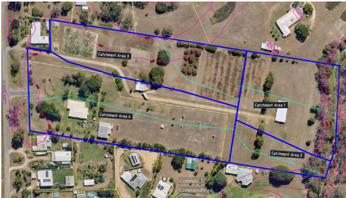
Figure 7: Pre-Development Stormwater Runoff
