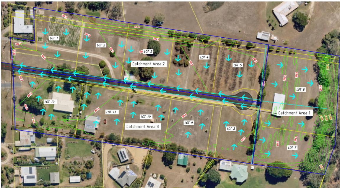
Figure 8: Post-Development Stormwater Surface Runoff
