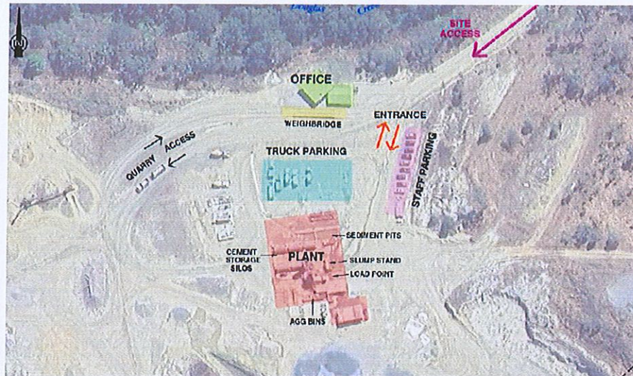
Figure 4: Concrete Batching Plant Operations: Site Layout.
