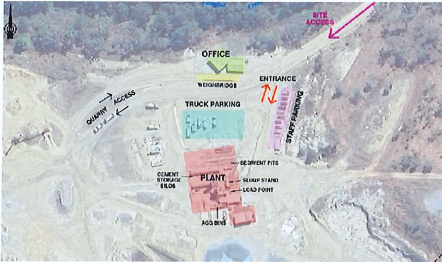
Figure 4: Concrete Batching Plant Operations: Site Layout.
