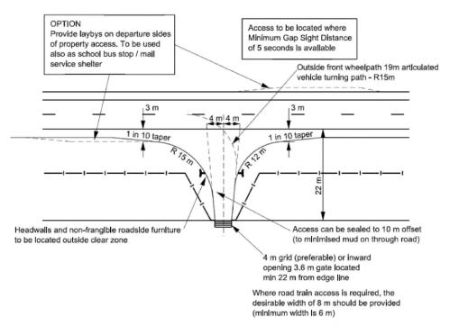
Note: Minimum requirement for a single carriageway with design AADT < 2000 or minimum requirement for dual carriageway left-in-left-out access for single unit truck. Where AADT > 1000 and access is required for a semi-trailer then use the layout.
