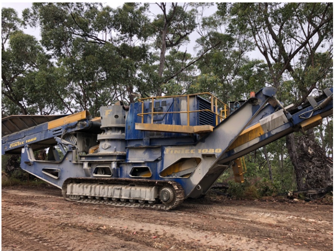
Figure 6: Finetec 1080 QH330 Sandvik cone crusher
