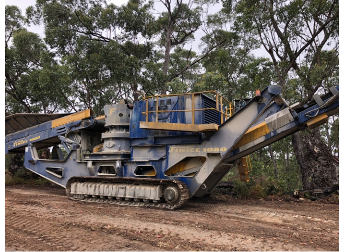
Figure 6: Finetec 1080 QH330 Sandvik cone crusher
