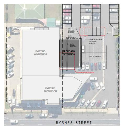
The workshop extension will have a gross floor area of approximately 236.6m2 and will facilitate the inclusion of an additional two (2) new hoists, three (3) detailing bays and a new tool room.
