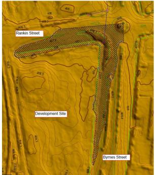
Figure 11 Potential Ponding Extent at Byrnes Street/Rankin Street Intersection
