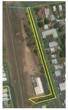
Figure 14 Catchment of the Kerb Inlet Pit on Western Side of Byrnes Street at the Byrnes Street/Herberton Street Intersection
