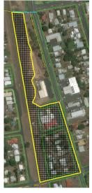
Figure 16 Catchment of Culvert Crossing under Abandoned Railway Formation
