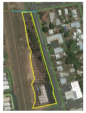
Figure 15 Catchment of Headwall (Table Drain) on Western Side of Byrnes Street at the Byrnes Street/Herberton Street Intersection
