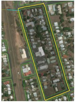
Figure 12 Catchment of the Kerb Inlet Pit on Eastern Side of Byrnes Street at the Byrnes Street/Herberton Street Intersection
