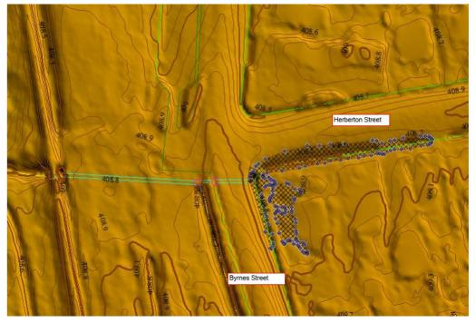
Figure 13 Potential Ponding Extent at Byrnes Street/Herberton Street Intersection
