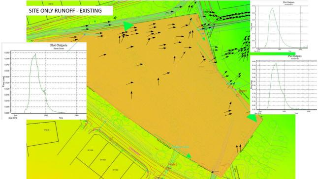
Flow lines indicating the existing site's discharge characteristics are shown in Figure 10.
