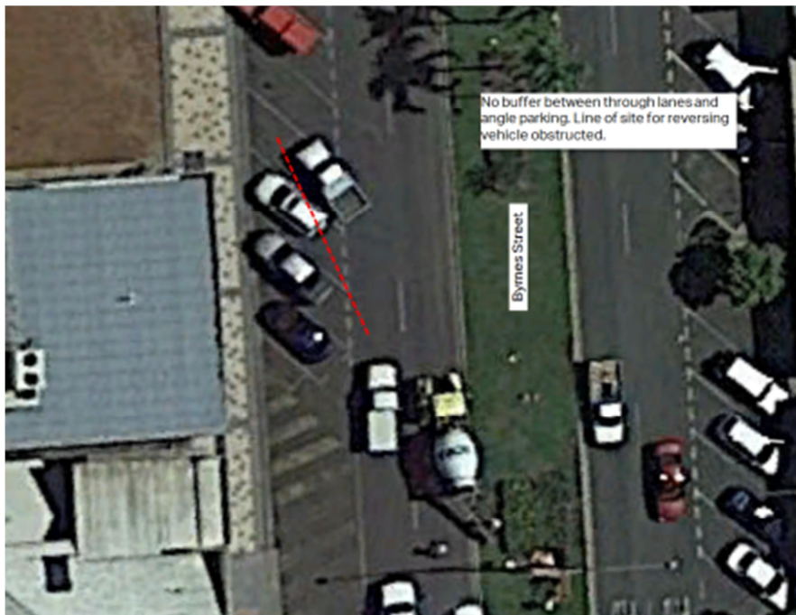
Figure 17 Byrnes Street – Line of sight for reversing from angle parking
